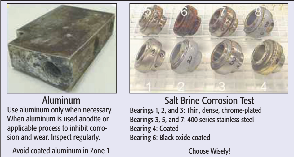
Figure 1. Principle 2: Made of Compatible Materials.
